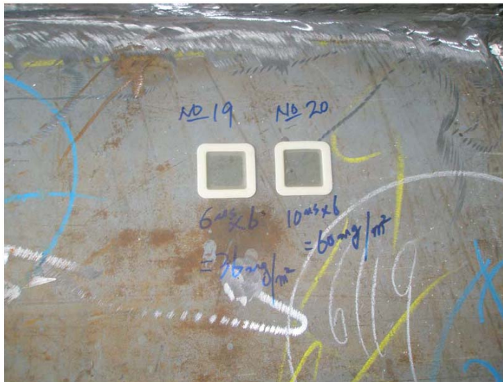
Block on an area with rust stain contamination over-head -Not expected to be contaminated by human traffic! Below, outer bilge area on the bottom plate.
