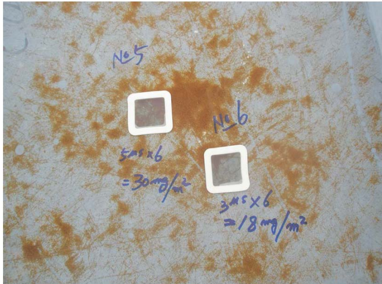
Above Panel I – Below Panel II 1 st pair – also horizontal washed in recent rains, on a heat weld damaged spot.
